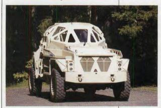
a blast bucket that helps deflect the energy of exploding mines. The result of this research is called the ULTRA AP. Office of Naval Research will now test the ULTRA AP to glean it for ideas that may be of use in future GI vehicles, and it is anticipated more will be built for field tests with mines and roadside bombs as well. Photo: U.S. Navy, by John F. Williams
